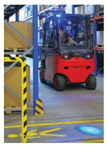
front of the forklifts. No matter what direction the truck is moving, there is a blue light to notify that a vehicle is approaching. Wolter added a blue light to the floor scrubber and a robotic stretch wrapper, making those two machines much more visible.
