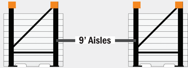
Compact/Reach Truck compared to a 4 wheel = 25% Space Savings
