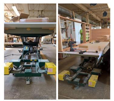
a highly efficient and flexible hydraulic scissor lift table by Southworth, called the Backsaver.
